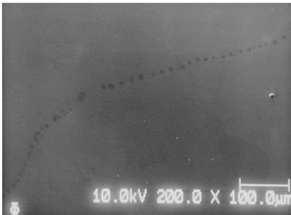
図 2 : [SC2] As machined surface with stained spots and a pit. Note the different scale comparing to the following figures.
